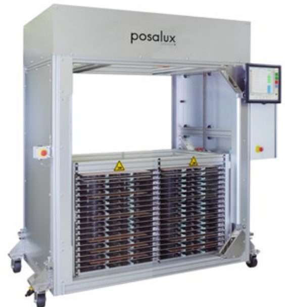
Individual loader (IL) with 9 or 18 levels
