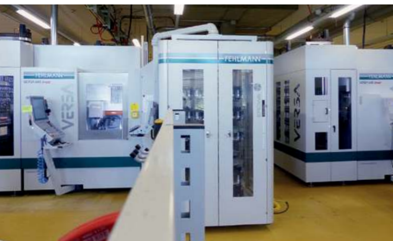
In 2018 the company invested in the first VERSA 645 linear 5-axis machining center, followed by the second in 2019. Both machines are connected with a Robot Multi (ERM) from Erowa.
