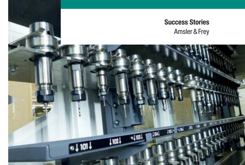
The set-up times were drastically reduced by the tool changer with a capacity for 200 tools.
